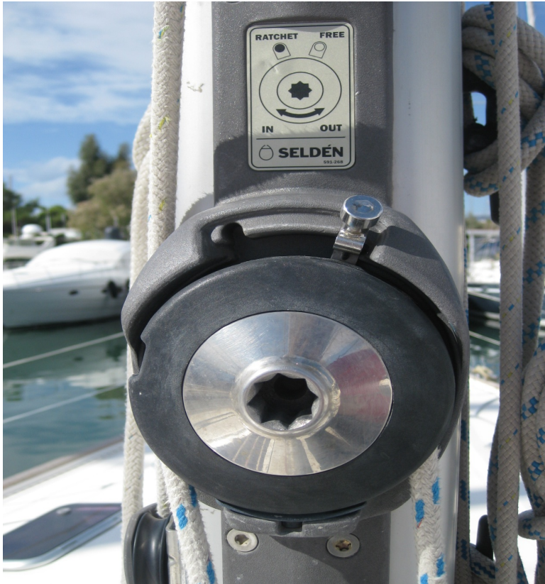
The winch on the mast that opens and closes the main sail, shown in photo in free position
