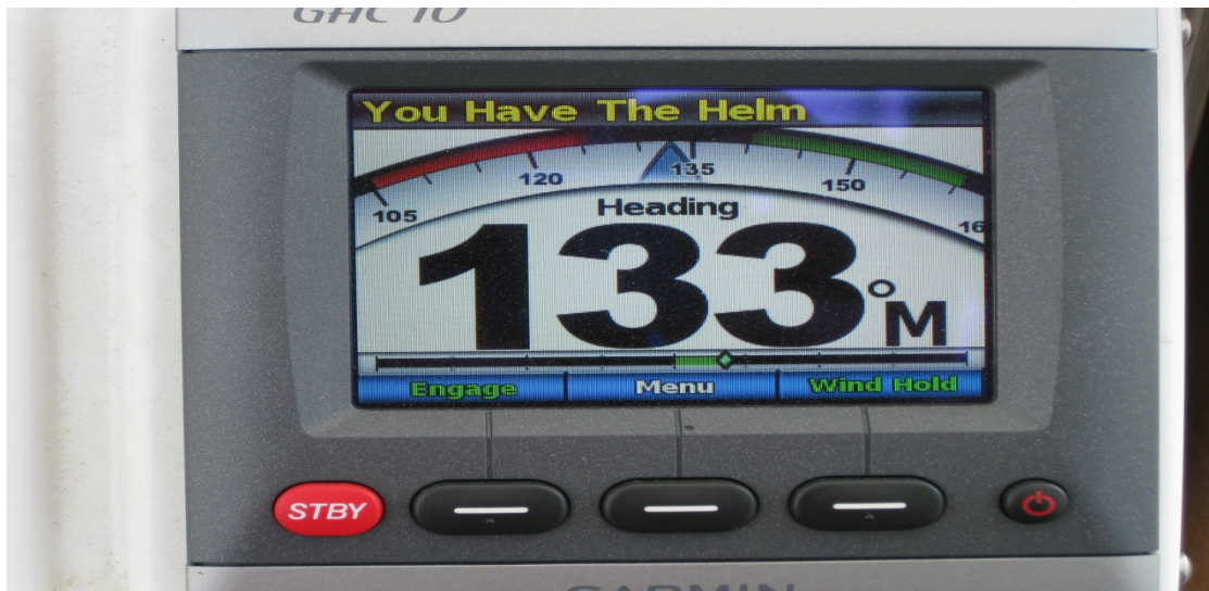
When you open the auto pilot instrument, you have to wait for 20 sec. Press escape when it will ask you for calibration.
