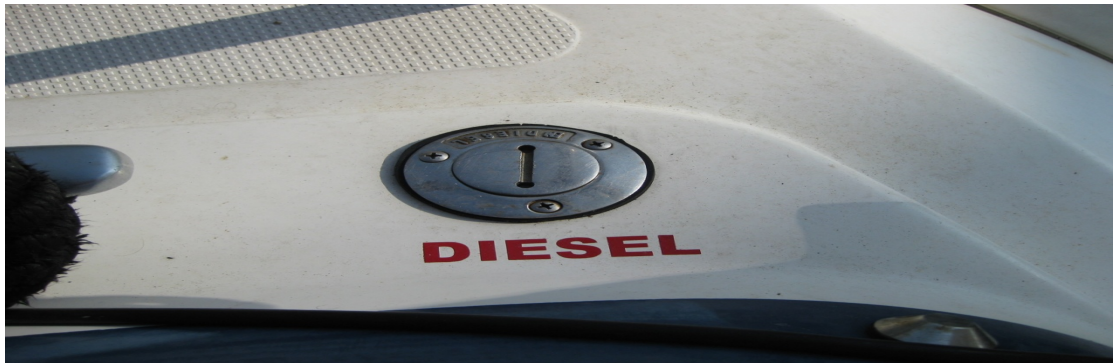
Diesel tap marked with red letters
